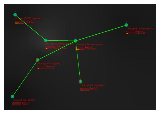
Each node was programmed to collect and send light readings every 10 seconds. The data was collected for 21 hours.
